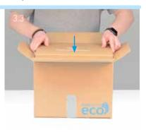
4. Set up the insulation ring, press firmly and insert
